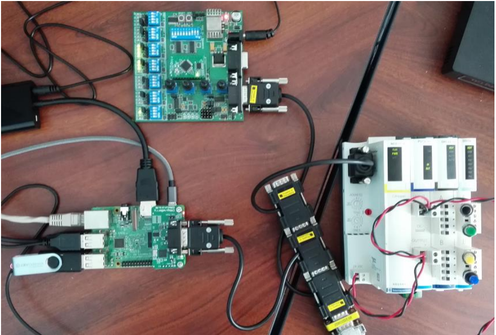
CANGINEBERRY WITH CANOPENIA-M0 AND SCHNEIDER ADVANTYS® SYSTEM
